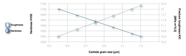
Vergnano carbide taps are produced in K grade carbide. The carbide grain size is "ultra-fine" (UF) which guarantees excellent hardness and toughness.
