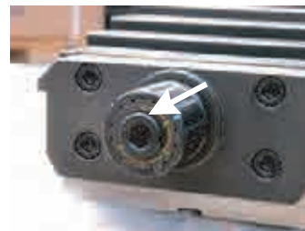
3. Release the adjustable knob to lock in the setting.
