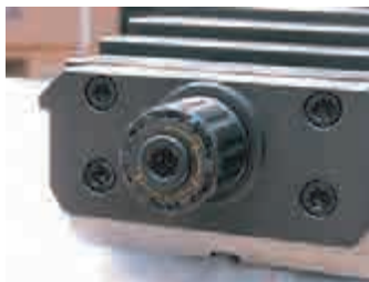
2. Rotate the adjustable knob to the required torque setting.
