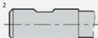
DIN 1835 B/DIN 6535 HB up to \varnothing 20 mm
